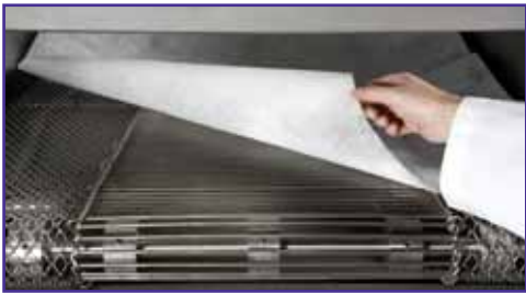
Fines are captured on filter paper and automatically removed from the filter.
